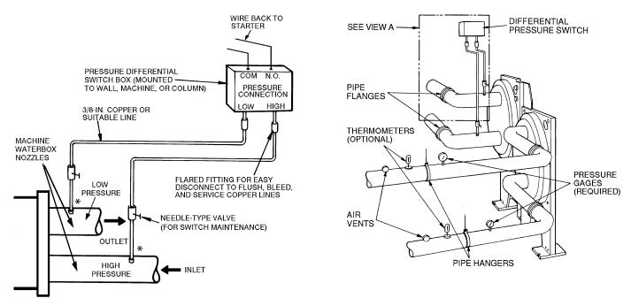
Fig. 19 — Typical Nozzle Piping
